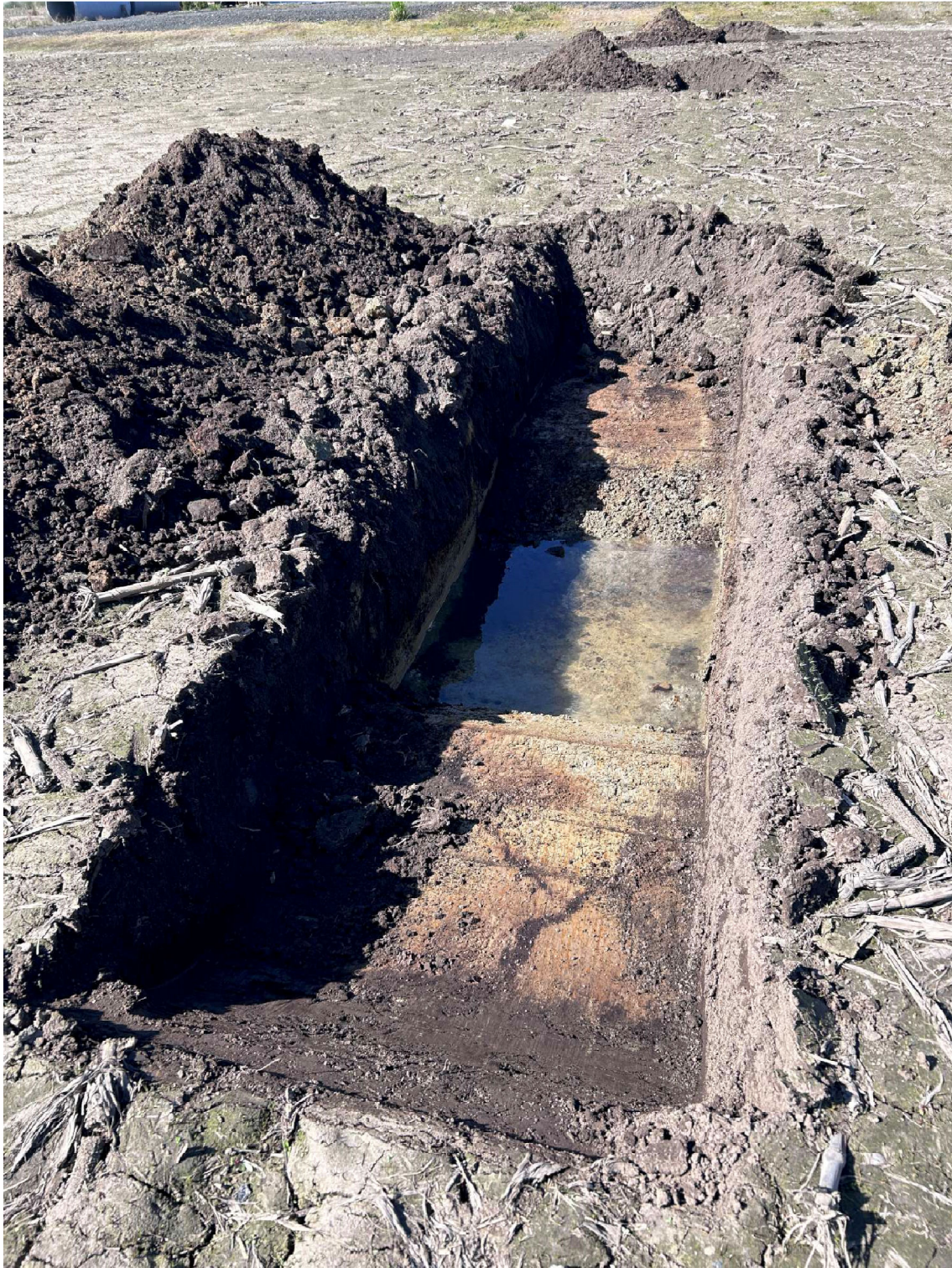
Typical shallow test pit into native clay with ponded water
