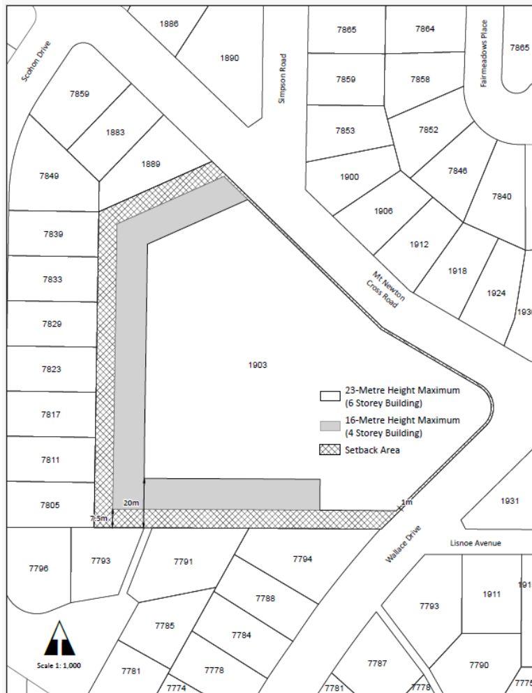
Figure 1: Building height allowances and surface parking area
